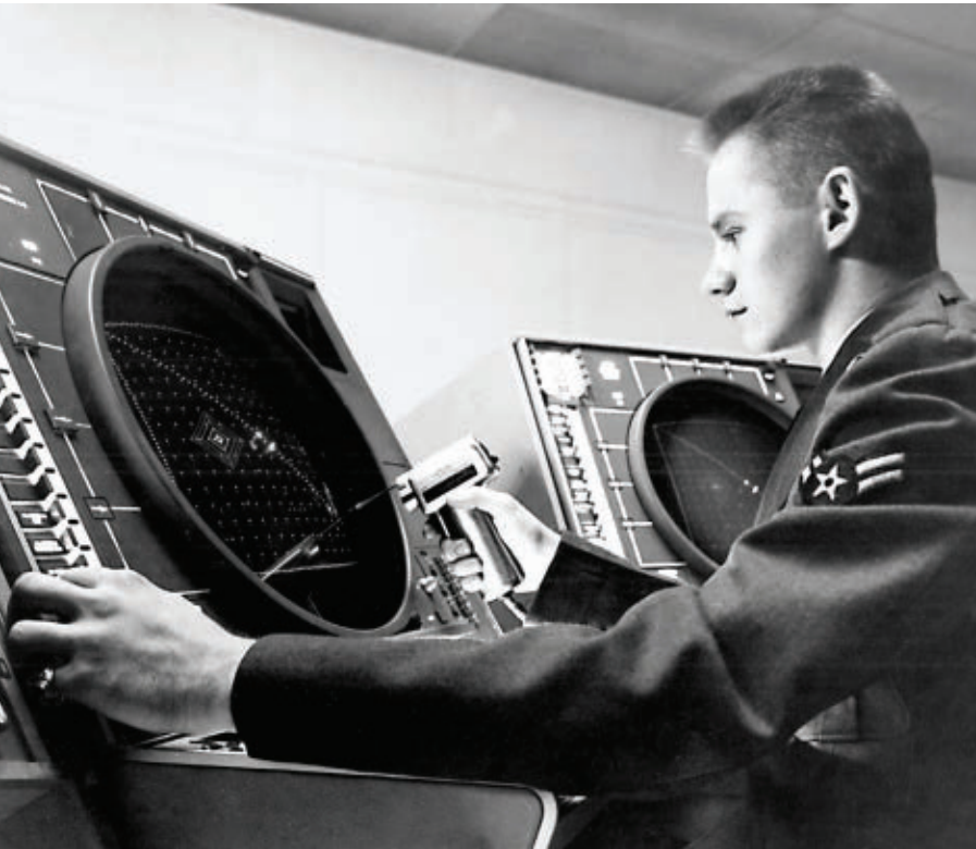
► A late 1950s SAGE console with "light gun" used to select radar tracks for display on central "summary board" (not shown). The operator accesses information and directs action using sliders, switches, buttons, and dials. Courtesy IBM Archives.
