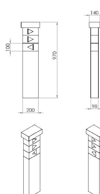
All guideposts have the same concretebase and they are designed to be modified with different materials.
